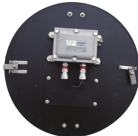
Figure 1. Underneath of a sensor node. Visible are the composite manhole cover, the explosion proof box containing all the electronics, a cam-lock system to maintain the lightweight cover in place, and the antenna (under the explosion proof box).
